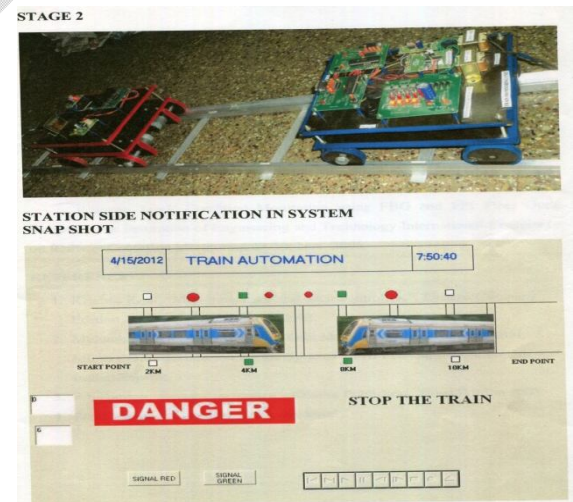
Fig 10 : Collision between the trains discarded by the MECE (Stage-2)
